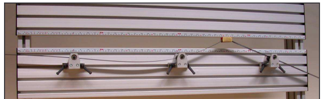
Fig. 4b. Influence line for bending moment at a section of a two-span continuous beam
