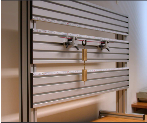
Fig. 1. Didactic test frame for structural mechanics
