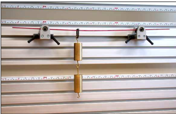
Fig. 2a. Test of a simply supported beam
