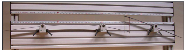
Fig. 4a. Influence line for shearing force
